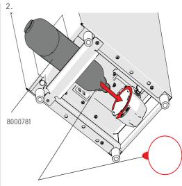
The orientation indicator on the filter should point left before rotating
